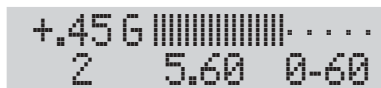
Showing acceleration of .45G, and a second-best top 0 to 60 run to date of 5.60 seconds.
