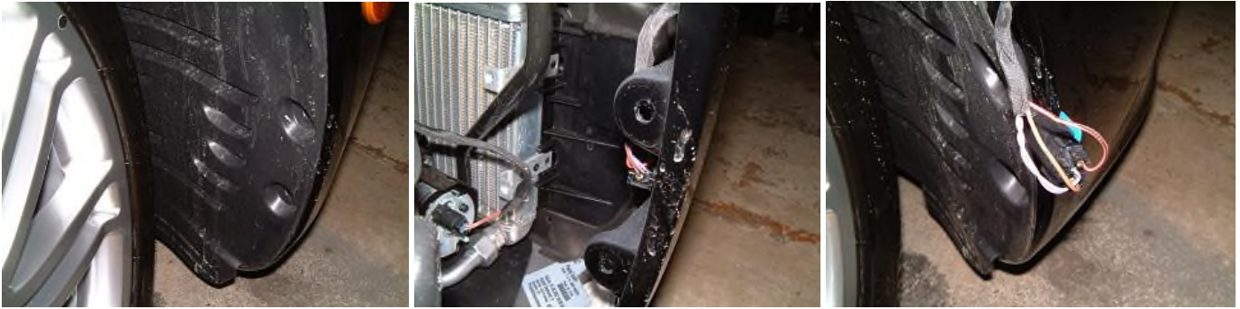
Front Wheel Well DISTRONIC Harness Location
